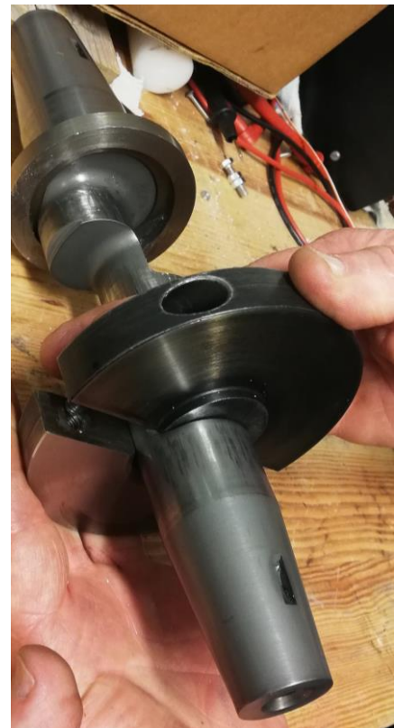
Figure 43. Guiding ring in the new crankshaft
