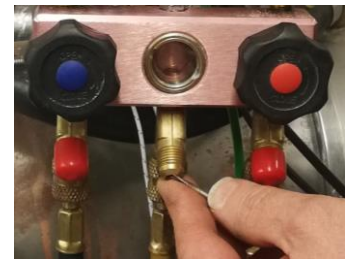
Figure 40. Evacuating air from the yellow hose
