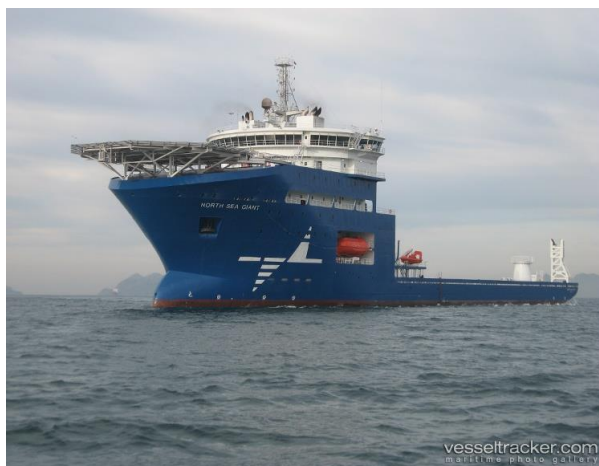
Figur 5. North Sea Giant, helikopterplattform under broen
