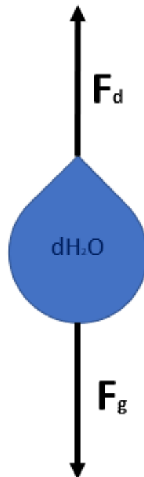
Figure 2.9 Graphic representation of the terminal velocity principle, where drag forces is equal to gravitational forces. Figure adapted from (Hall 2015).
