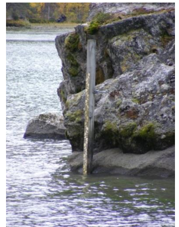
Fig. 35 Example of measurement pole at Straumavatnet to measure the water level
