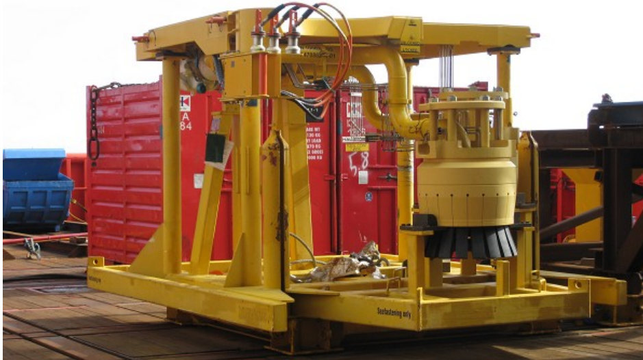
Photo 6: Subsea Control Module
