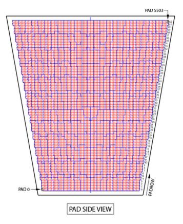
Figure 2.4: Pad structure of an Inner Readout Chamber(IROC)[15].
