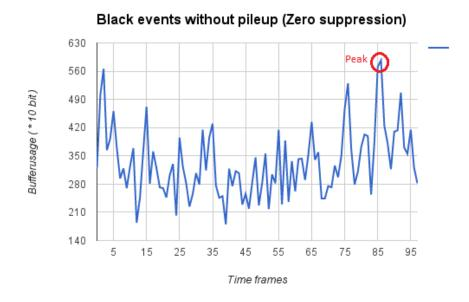
Figure 6.14: Results from Black events w/o pileup using Zero suppression.
