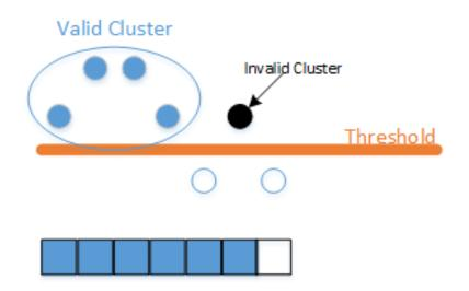
Figure 5.1: An edge case that the Zero suppression needs to handle.
