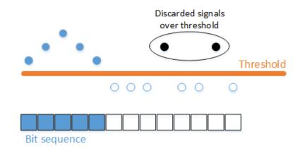
Figure 4.4: Difference between a valid and invalid signal sequence.
