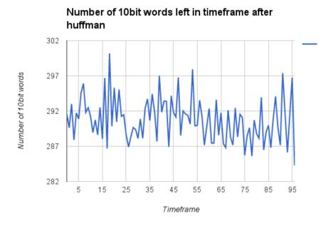
Figure 6.22: Results from using Huffman encoding on simulated RUN 3 data.
