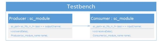
Figure 3.1: Basic SystemC example.
