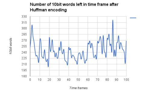
Figure 6.16: Results from Black events w/o pileup, using Huffman encoding.
