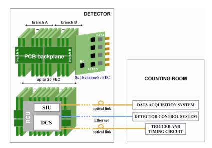
Figure 2.3: Readout schematics for the current TPC detector [14].
