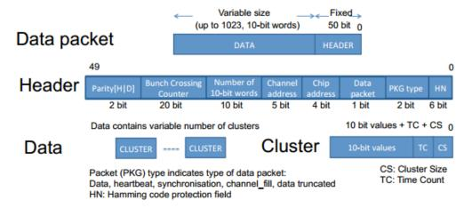
Figure 4.2: Data packet format [16].
