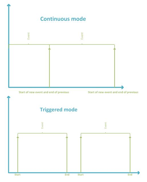
Figure 4.1: Continuous vs Triggered mode.
