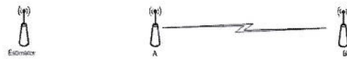
Figure 3 – Scenario 3, chain topology, with node B sending traffic towards node A, estimator node outside of node Bs range. Estimator is sending probes to node A.
