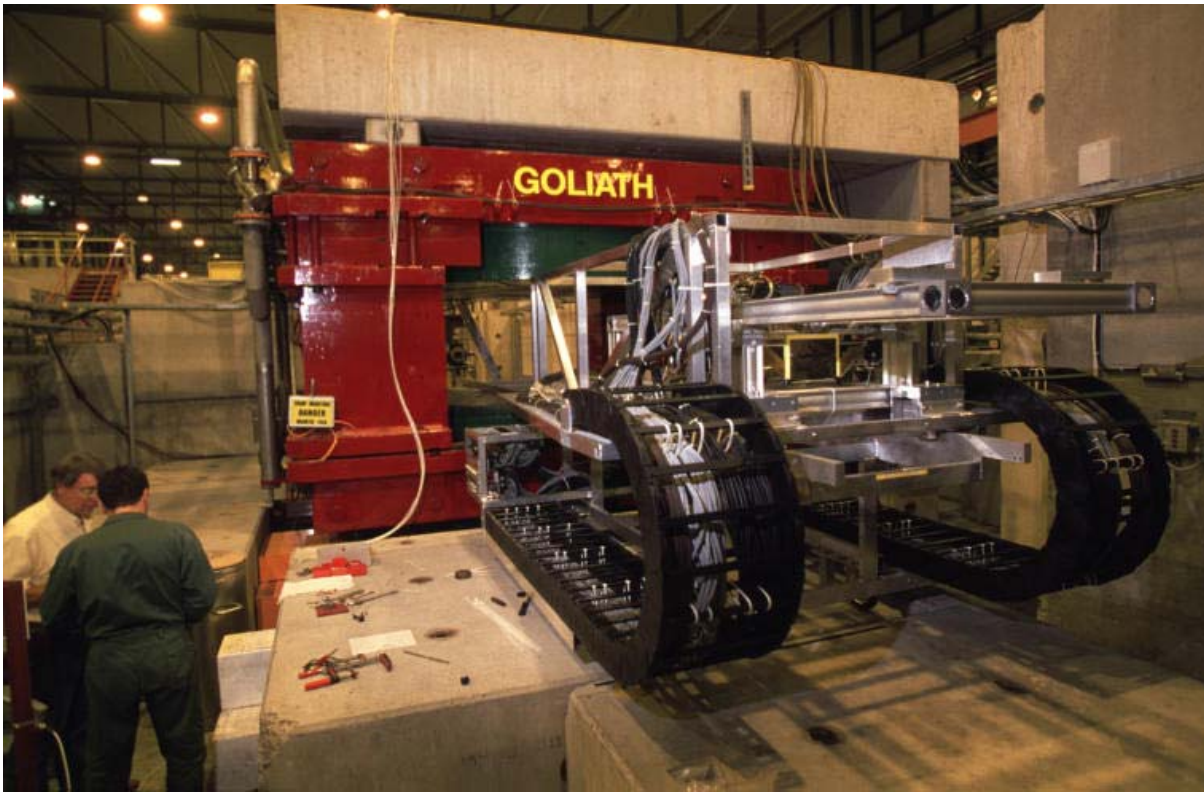
Figure 2.7: The GOLIATH magnet with the silicon telescope mounted on rails.
