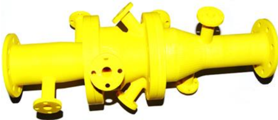
Fig. 2.82.FDM prototype of jet pump
