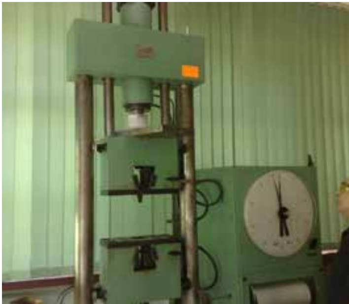
Fig. 4.6. View of universal testing machine
