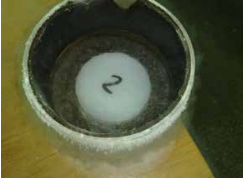
Fig. 4.7. Cooling of the sample in the calorimeter
