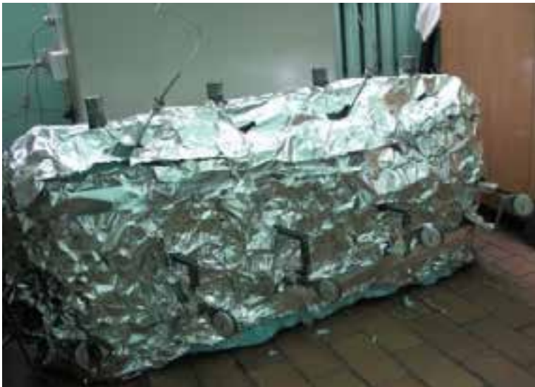
Fig. 4.2. View of laboratory test stand: a) before insulating b) with full insulation during the tests
