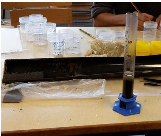
Figure 2a In the front is a measurement cylinder for the volume measurement. Behind is a core and in the very back are some cups to store the sediment in.
