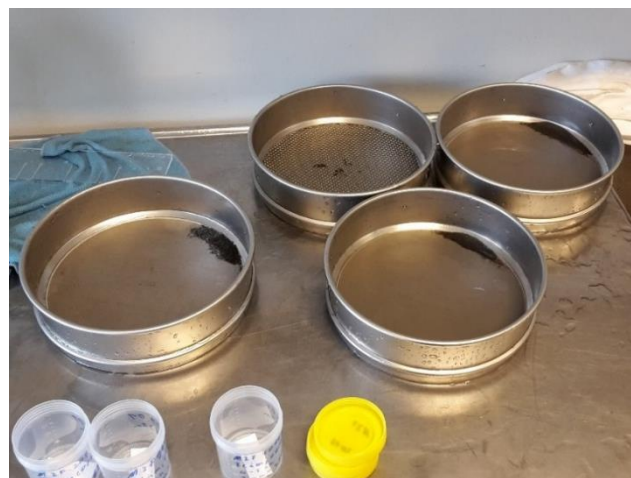
Figure 2b The four sieve sizes with the remaining sediments for each size fraction
