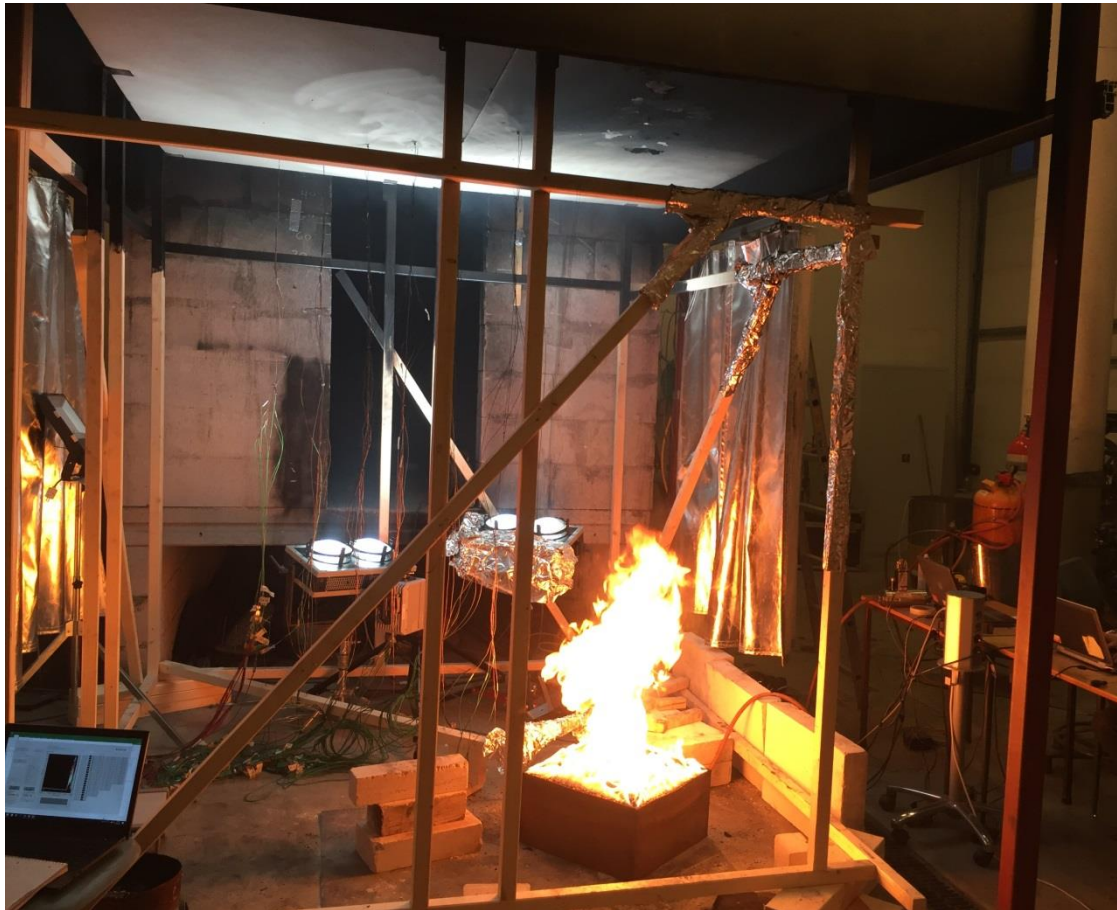
Figure 12 Picture of the experimental setup in the laboratory. The fire has a heat release rate of 80 kW, under a ceiling height of 2.39 m. To left of the fire the arrangement of thermocouples can be seen hanging from the ceiling.
