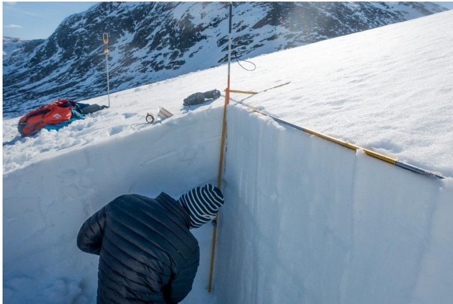
Figure 3.1. Emil Solbakken records the snow temperature after excavating the side wall at the study site at Strøngeskaret. Photo: Åsmund Karlsnes.
