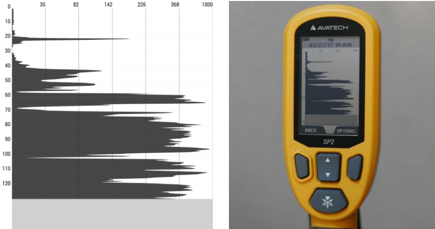
Figure 3.7. SP2 hardness profile as shown on Avonet (left) and on the built-in screen (right).
