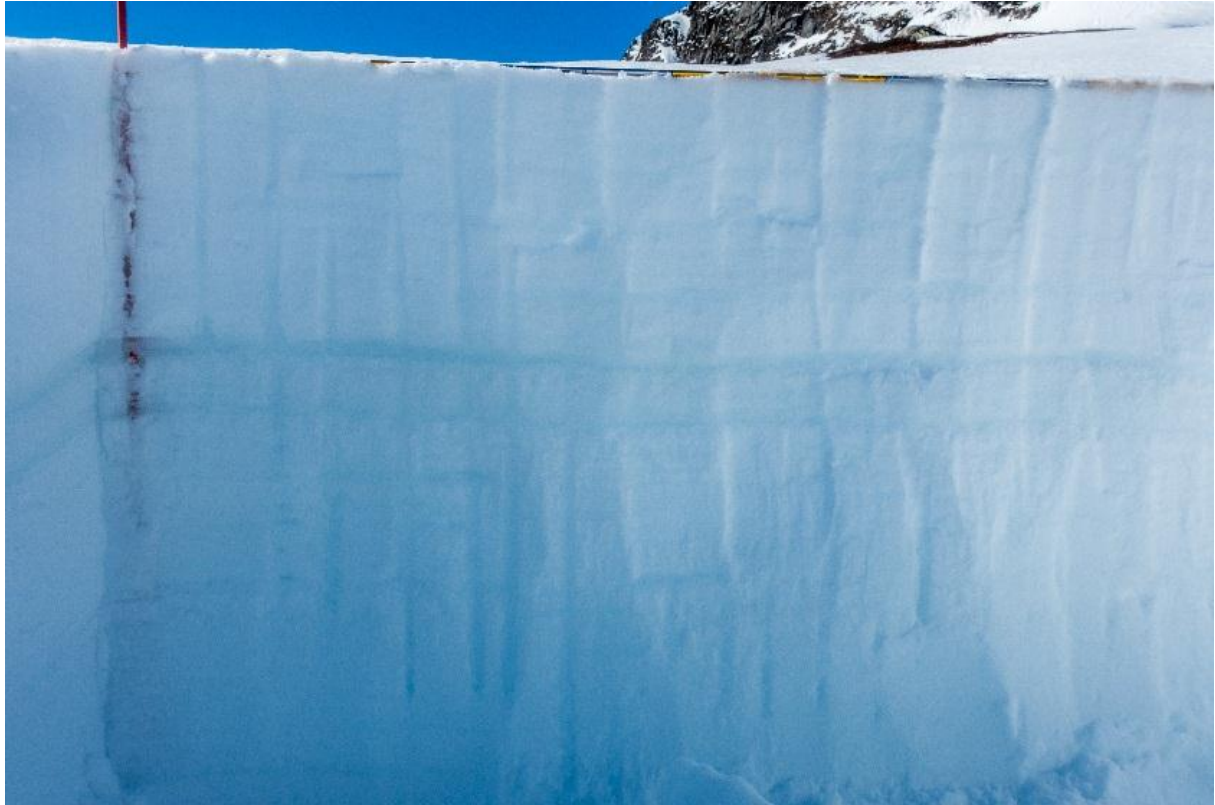
Figure 3.5. The back transect wall at the Hemsedal 2 site at Strøngeskaret. The vertical lines in the snow are the probing holes made during SP2 probing. Photo: Åsmund Karlsnes.
