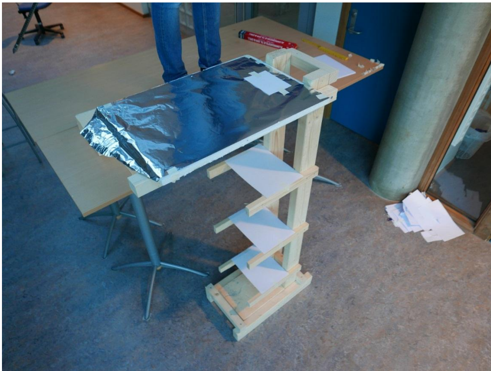
Figure 3.6. The construction used to test the depth accuracy of the SP2 in the lab. The printer papers work as resistance layers. The tinfoil is used as a reflector for the IR-sensor. Photo: Emil Solbakken.
