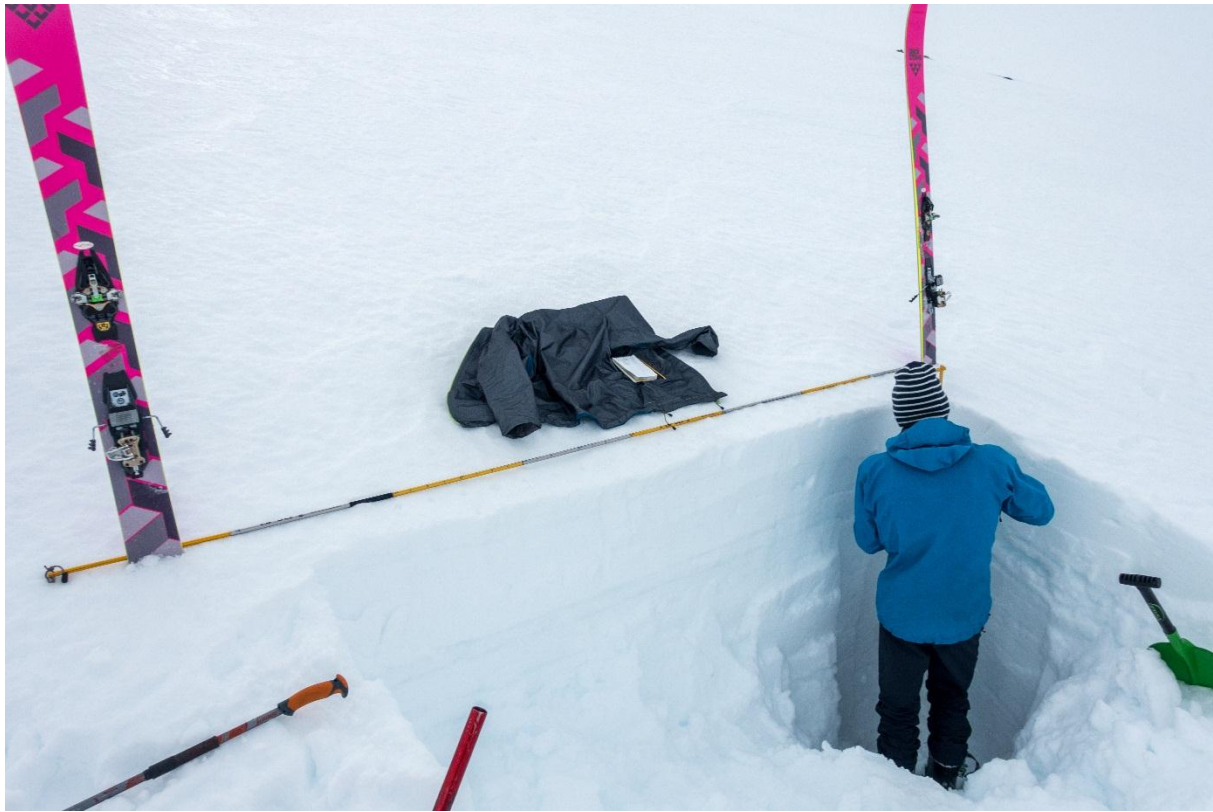
Figure 5.1. A typical transect setup under excavation. The penetrometer tests were done along the avalanche probe. The picture is taken at the Filefjell 2 test site. Photo by Åsmund S. Karlsnes.
