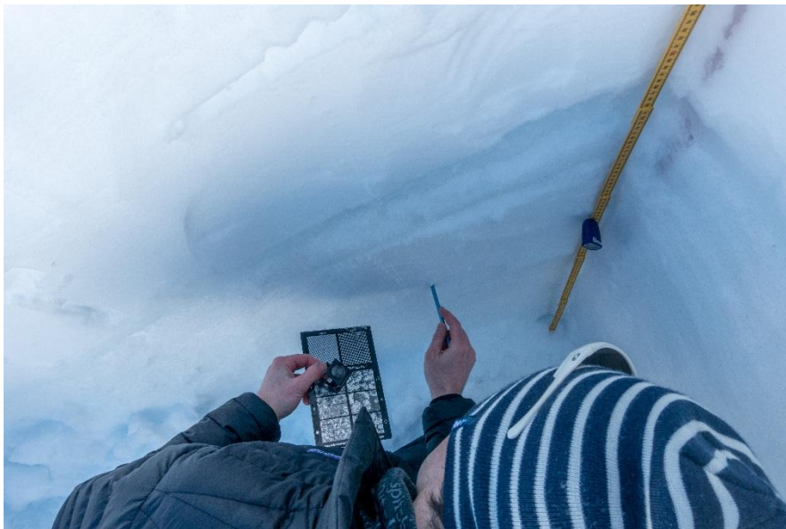
Figure 3.2. Emil Solbakken during layer identification at the Hemsedal 2 study site. Layer identification was done on the side wall of the transect. The ruler was used to measure depth.
