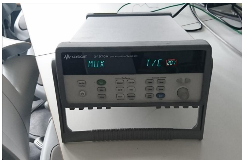
Bilde 8 - Datalogger, Keysight 34970A Data Acquisition
