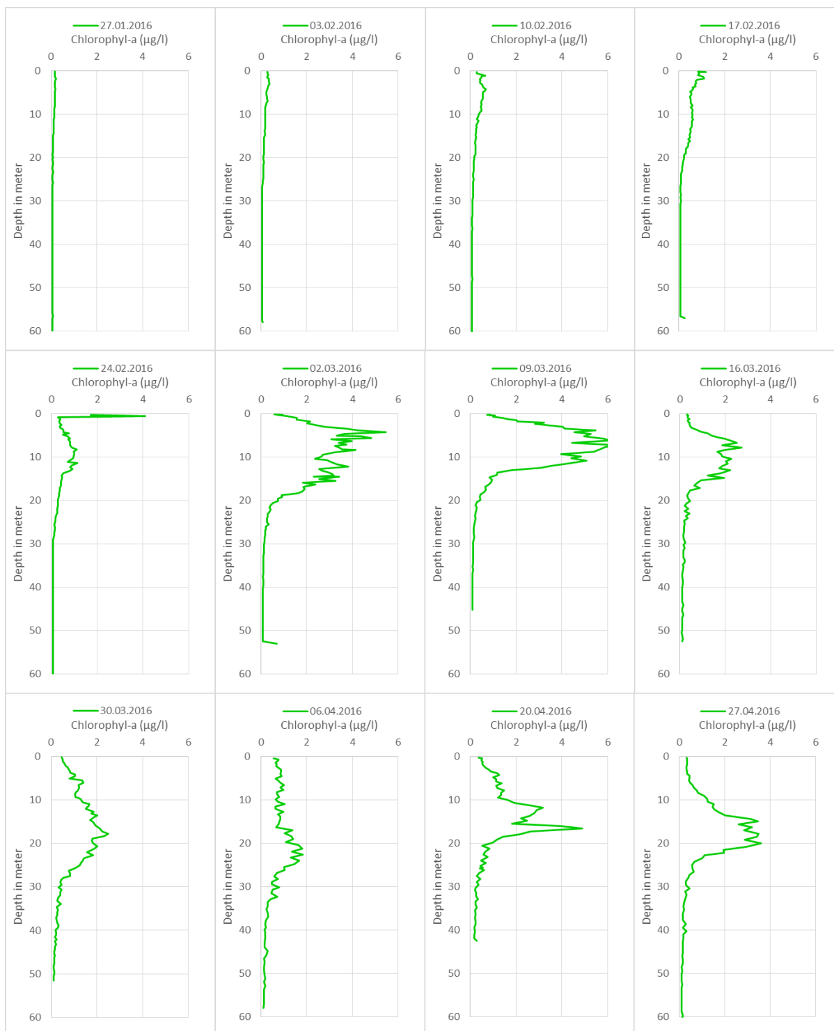
Figure 35 Chlorophyll- a time series per measurement date. The highest values are found on March 9 th , with concentrations reaching approximately 8 \mu\text{g/l} at a depth of seven meter. This peak is not shown in the figure
