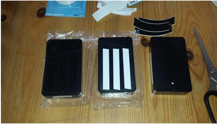
Figure 4: The process of attaching double adhesive tape and Velcro strips to the back of the receivers and transmitters.
