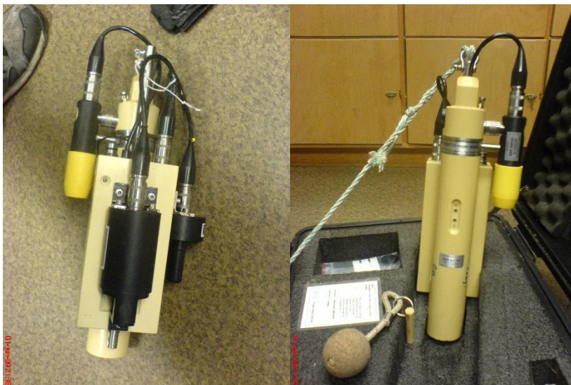
FIGURE 8 CTD-DEVICE (SAIV 204) PICTURE ON THE RIGHT WITHOUT TURBIDITY SENSOR (KILDE T. DALE)
