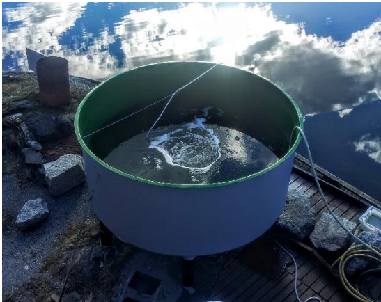
FIGURE 2 TANK DURING REFILL, FOAM FROM AERATION VISIBLE ON THE SURFACE
