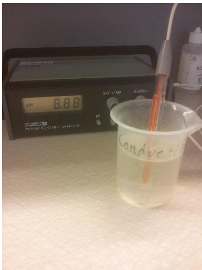
FIGURE 124 PORTABLE PH-METER (RADIOMETER: PHM 80)
