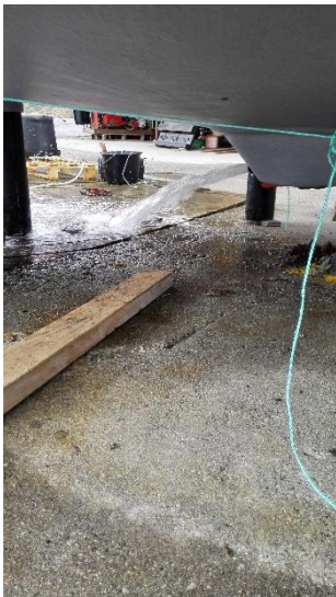
FIGURE 3 TANK (BOTTOM) WITH LEGS AND DRAINING VALVE
