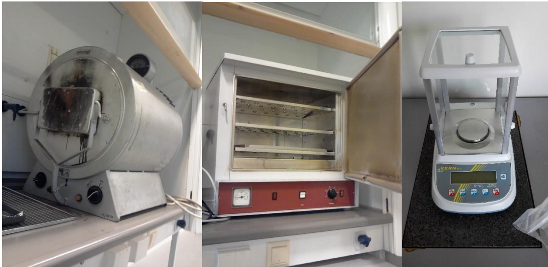
FIGURE 12 FROM THE LEFT: MUSSLE OVEN (HERAEUS MR 170), DRYING OVEN (TERMAKS T1056V), WEIGHT (KERN ALJ-1604A)
