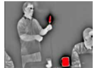
Hot Spot Detection set to alert >93° C (200° F)
