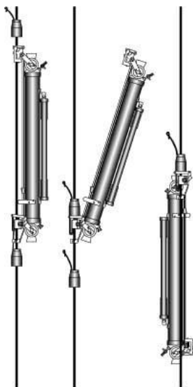
Figure 14: Nansen water bottle before, during and after reversing. (oceanworld.tamu.edu, 2015)
