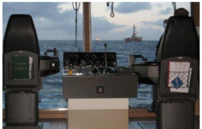
Picture 5: The bridge – winch is handled from the left chair, the vessel from the right
