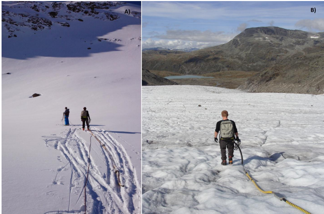
Figure 8: Application of GPR during the accumulation season (A) and ablation season (B), with a 50 MHz and 100 MHz antenna respectively.
