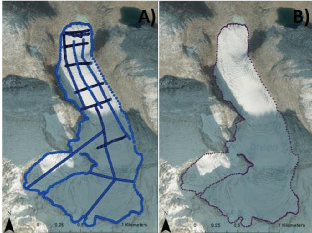
Figure 26: Boundary, interpolation profiles and profiles surveyed in the field (A). Glacier boundary, with depth equal to 0 (B).
