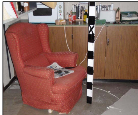
FIGURE 1: THE EASY CHAIR THAT WAS USED AS INITIAL FIRE IN THE FULL SCALE TEST.
