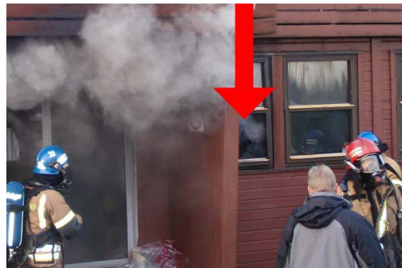
FIGURE 20: PICTURE FROM THE FULL-SCALE TEST WHERE THE ACTUAL VENTILATION THROUGH THE WINDOW CAN BE OBSERVED.
