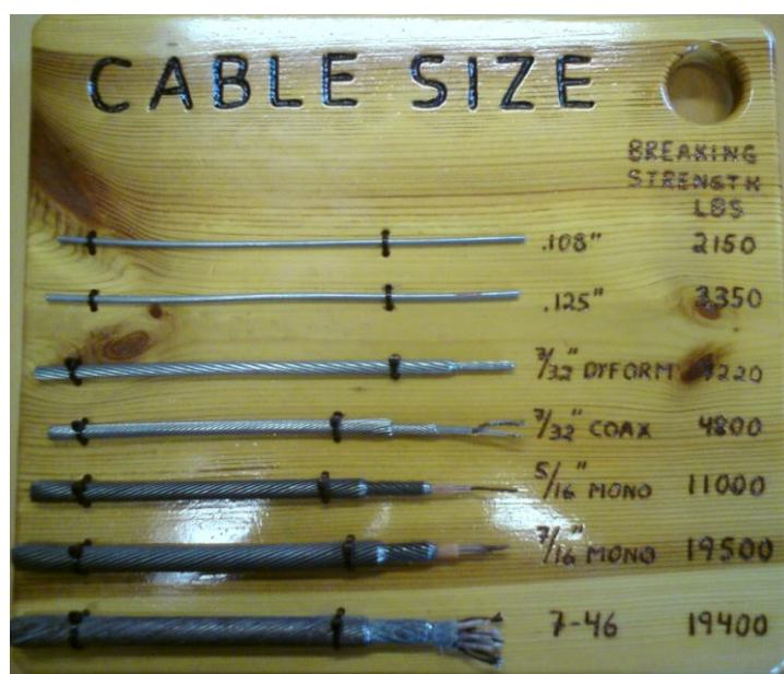
Figur 1: "Braided line" & "Slickline" kabler
